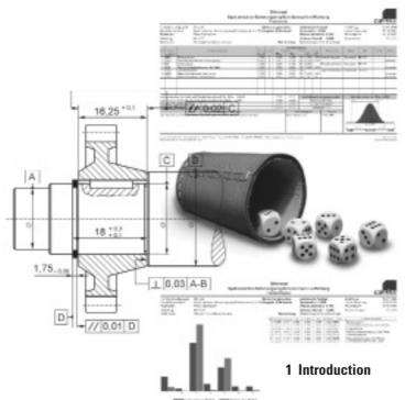
Tolerance analyses are indispensable to prove the technical practicability of sub-assemblies under mass production conditions. This contribution is intended as an attempt to show an empirical resolution method which allows the easy implementation of complex tolerance analyses on arbitrary physical systems.
